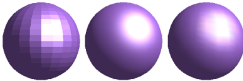
An identical mesh rendered using the Flat, Phong, and Gouraud lighting models, respectively.
